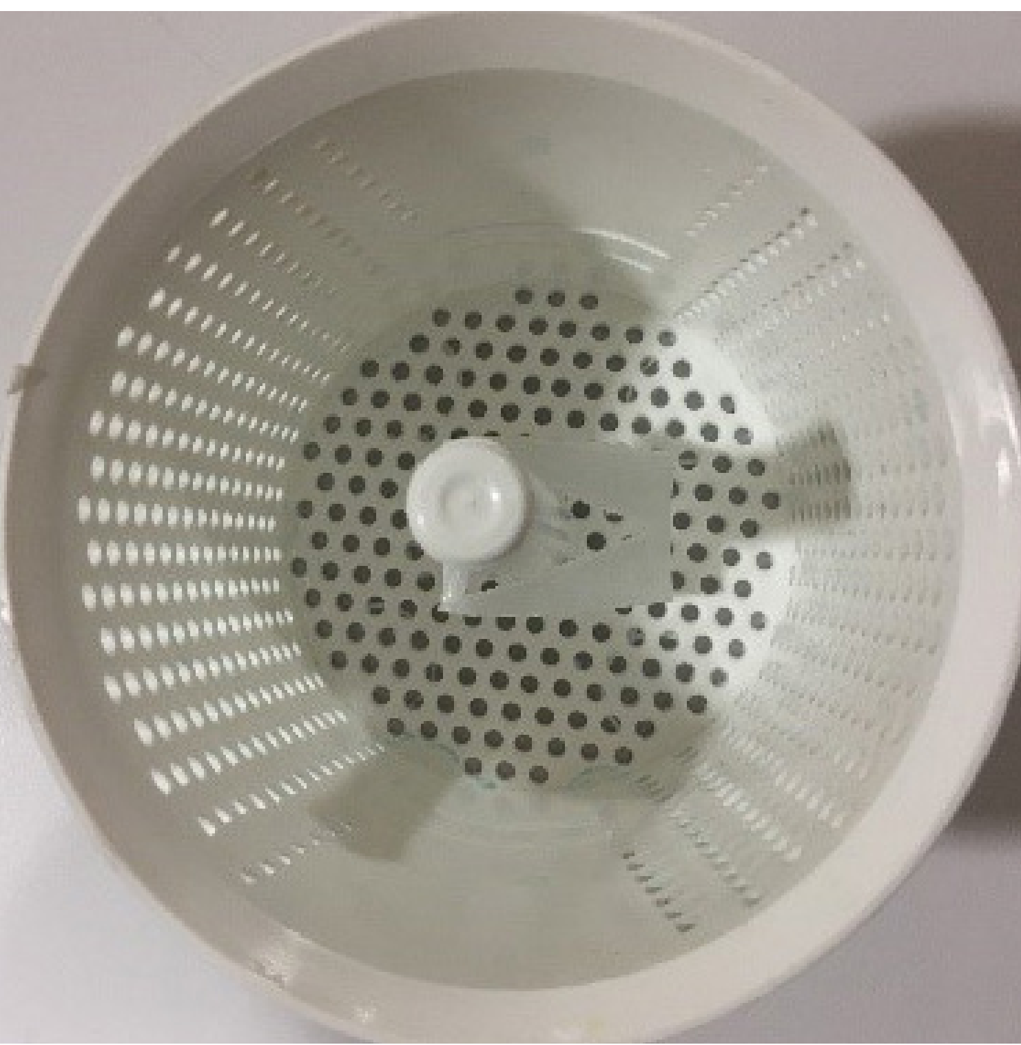
Figure 2: Apivar® strip (including the V-shaped opening) attached to the white basket of the Varroa EasyCheck® device.
